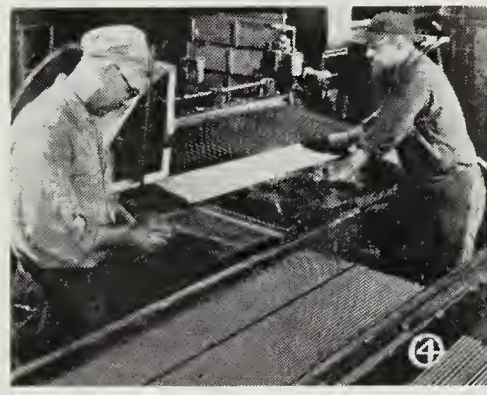
Fig. 3—Hallow carbon arc comes from hydraulic press, which extrudes blend material. Fig. 4— Arc carbons are precision cut into lengths for additional processing. Fig. 5—Skilled hands place the arc carbons into saggars packed with coke to support them during the oven baking.
